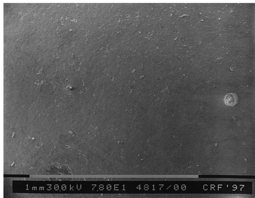
Fig. 6. Scanning electron micrograph of the CA coated SiC/SiC CVI surface after the compatibility test with Li 4 SiO 4 at 800°C for 140 h.
